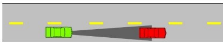
ACC reduces the green car's speed and maintains the preset headway.
