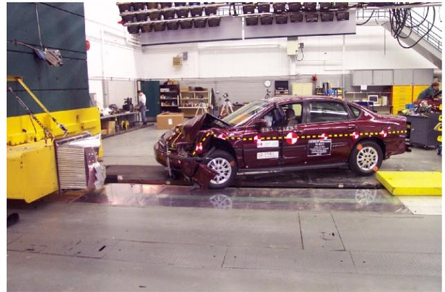
**Figure 2. Offset Deformable Barrier Crash Test**
