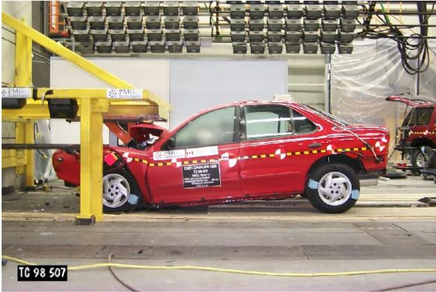
**Figure 3. Underride Guard Crash Test**
