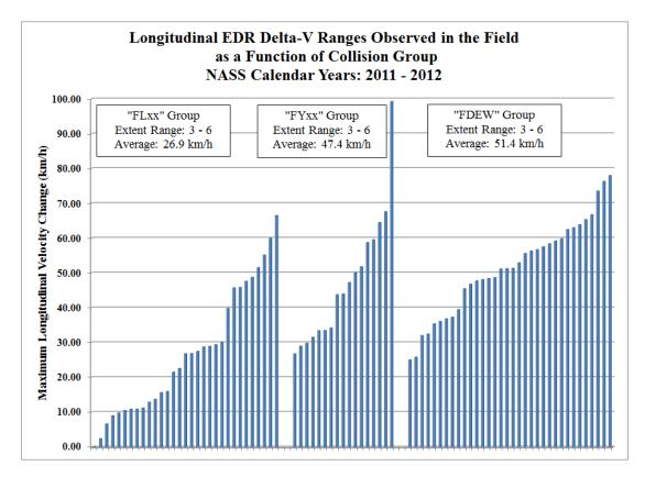
Figure 4. Longitudinal Delta-V in 2011-2012 NASS Cases
