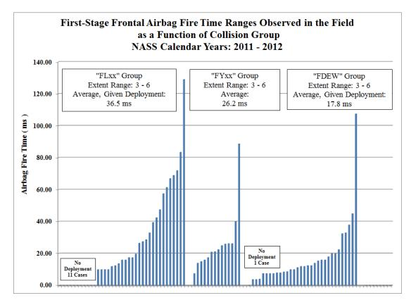
Figure 5. Frontal Airbag Fire Times in 2011-2012 NASS Cases
