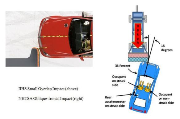
Figure 1. Small-overlap crash tests
