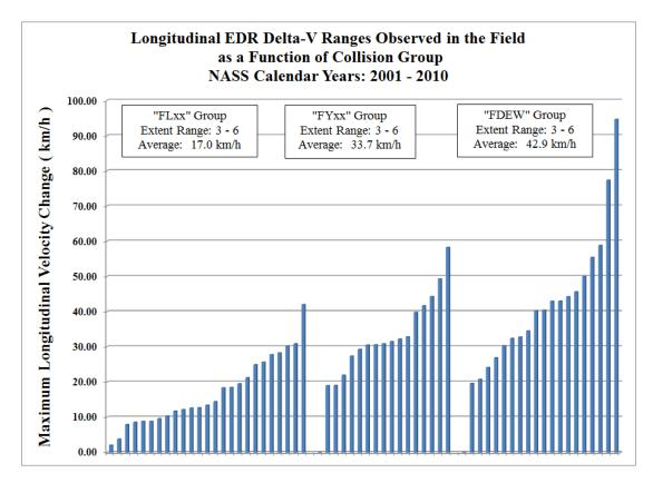
Figure 2. Longitudinal Delta-V in 2001-2010 NASS Cases
