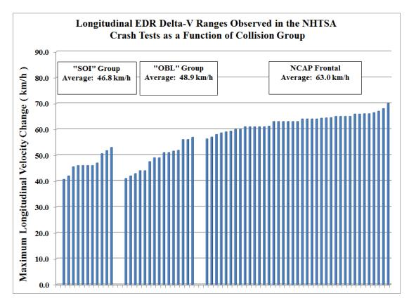
Figure 7. Longitudinal Delta-V in NHTSA Crash Tests
