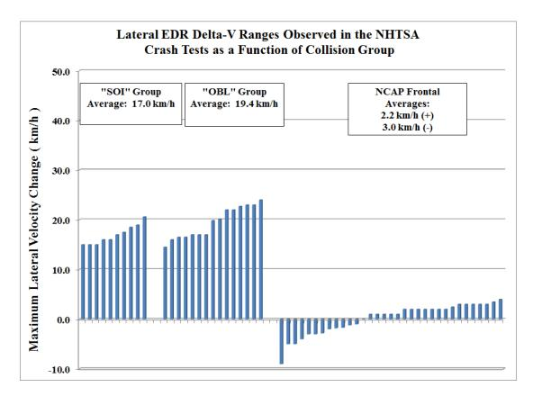
Figure 9. Lateral Delta-V in NHTSA Crash Tests
