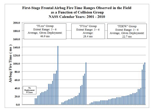
Figure 3. Frontal Airbag Fire Times in 2001-2010 NASS Cases
