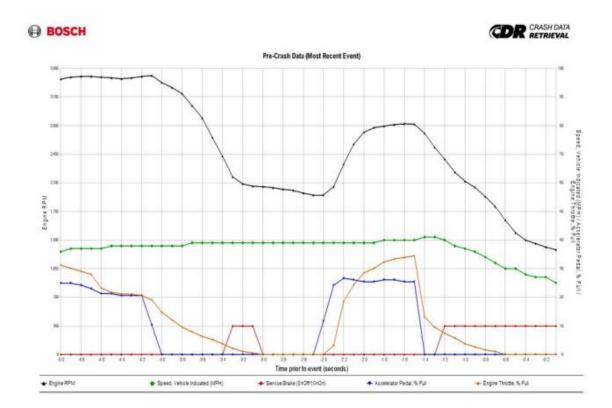
At 1.2 seconds prior to impact, the driver of the Journey applied the vehicle's brakes, holding them on until impact, as demonstrated by the approximately linear decrease in vehicle speed. The anti-lock braking system engaged for part of this time (one second to 0.5 seconds prior to the crash).
