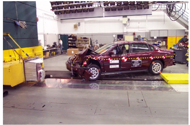
Figure 2. Offset Deformable Barrier Crash Test
