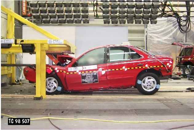
Figure 3. Underride Guard Crash Test
