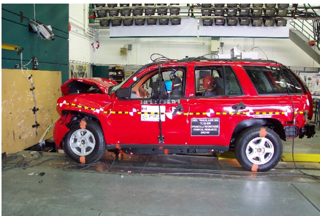
Figure 1. Frontal Rigid Barrier Crash Test
